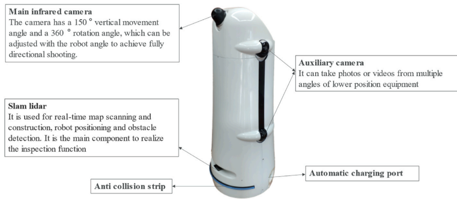
Fig. 13. Components of intelligent inspection robot.
