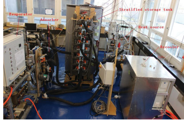
Fig. 3. The adsorption refrigeration system experimental platform.
