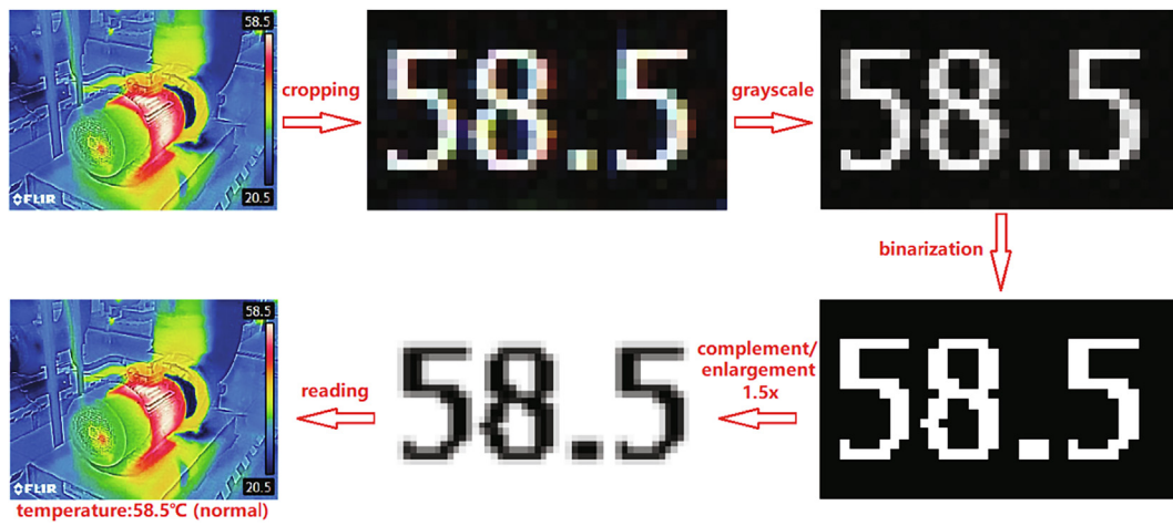
Fig. 20. Actual image processing flow and results.
