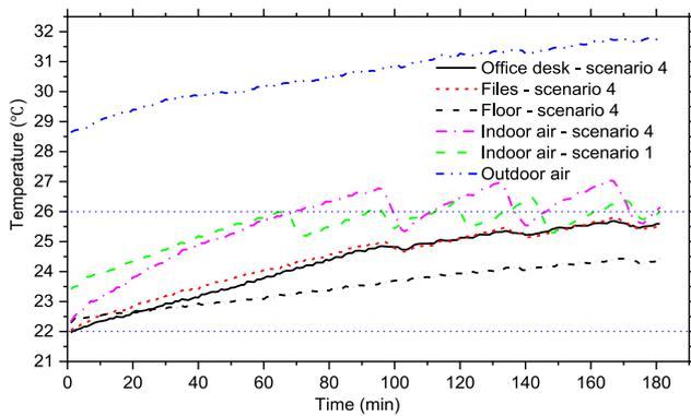
Fig. 6. Temperature variation of the pre-cooling control strategy.
