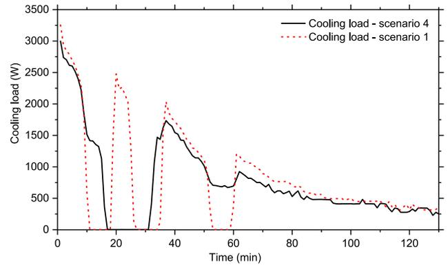
Fig. 11. Cooling load release curve of a storage tank.
