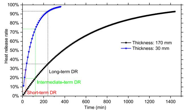
Fig. 13. Heat release rate of thermal mass of different thickness.
