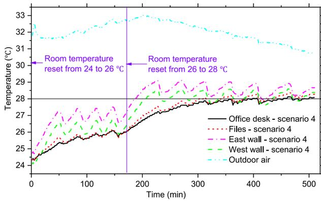
Fig. 8. Temperature variation for higher temperature resetting strategy.
