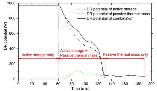
Fig. 12. DR potential combination (cooling release) of passive and active strategy in scenario 4.
