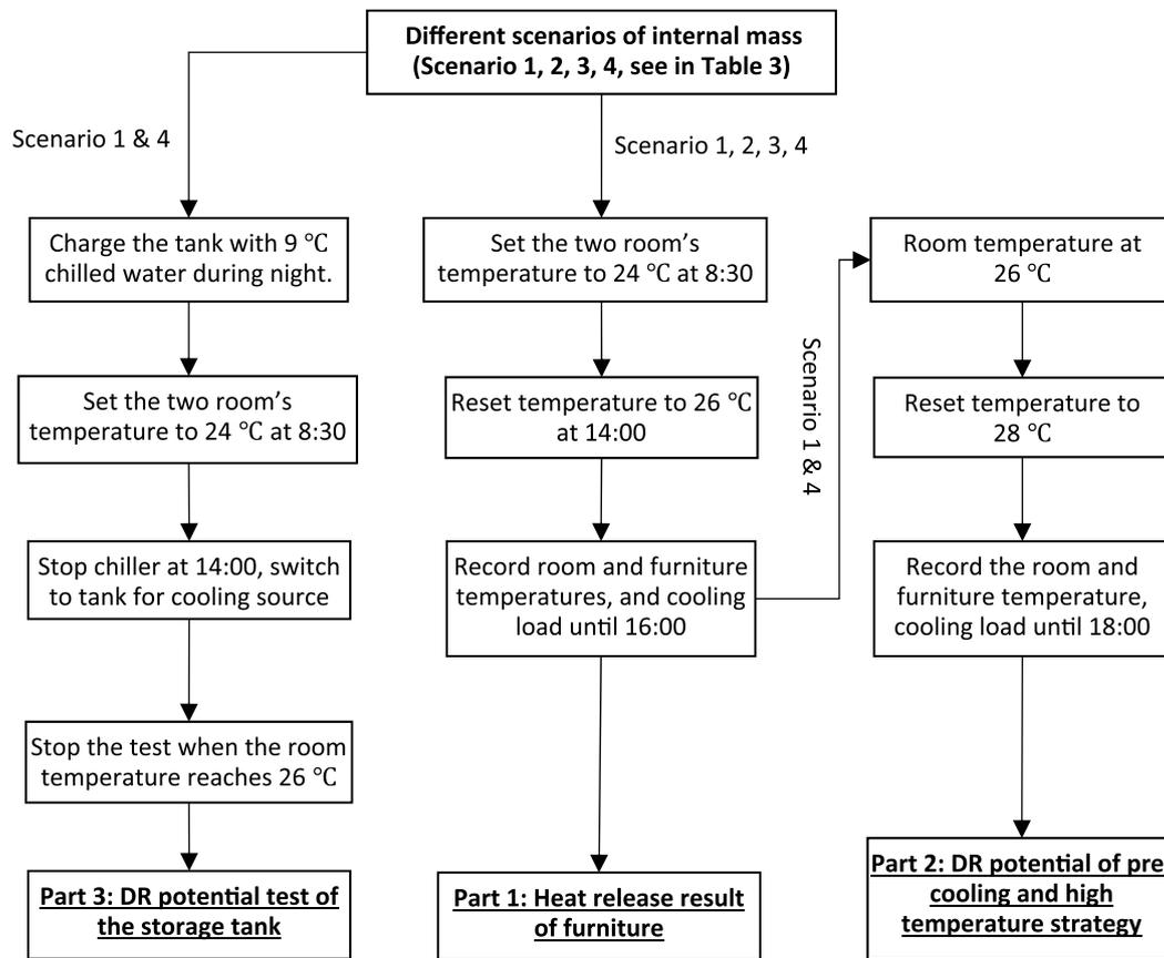
Fig. 2. Schematic of the experiment schemes.
