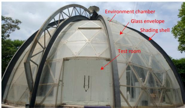
(b) Photograph of the environment chamber (Shading shell is open)
