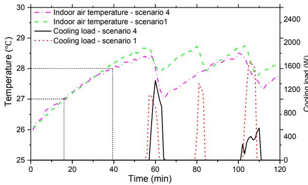
Fig. 9. Cooling demand for higher temperature resetting strategy.
