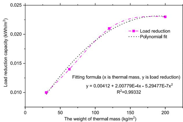
Fig. 14. Relationship between load reduction capacity and weight of internal thermal mass.
