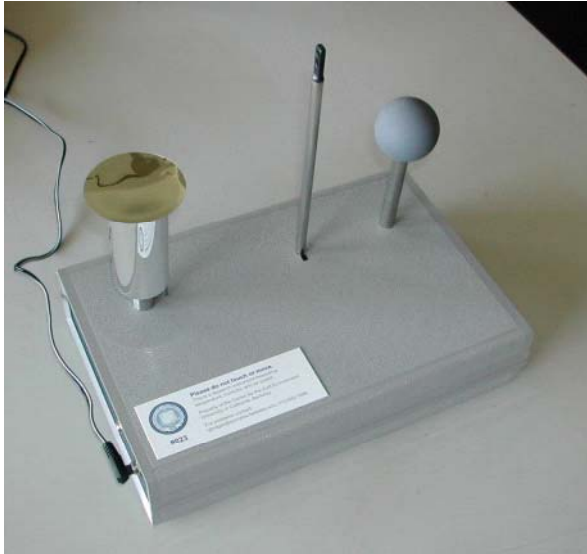
Figure 3. Indoor Climate Monitor (ICM) with (from left to right) shielded dry bulb sensor, anemometer (air speed sensor), and globe temperature sensor
