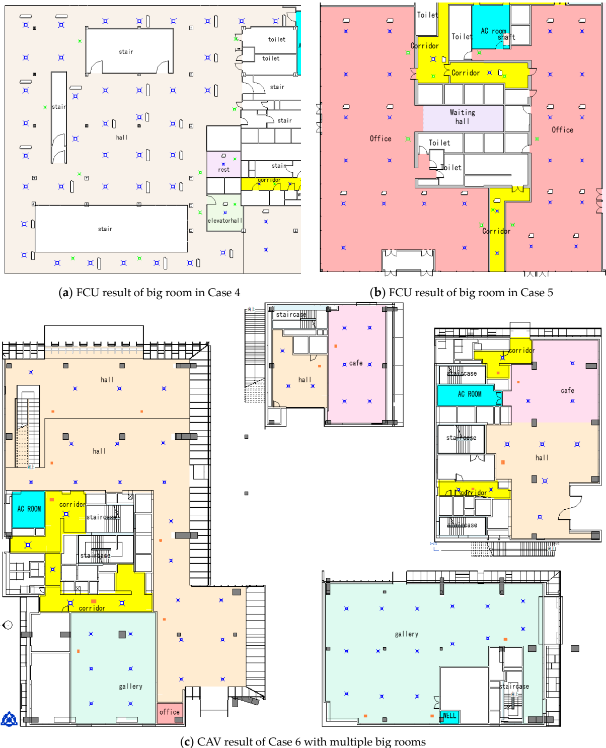
Figure 12. Placement result in big rooms of Cases 4–6.
