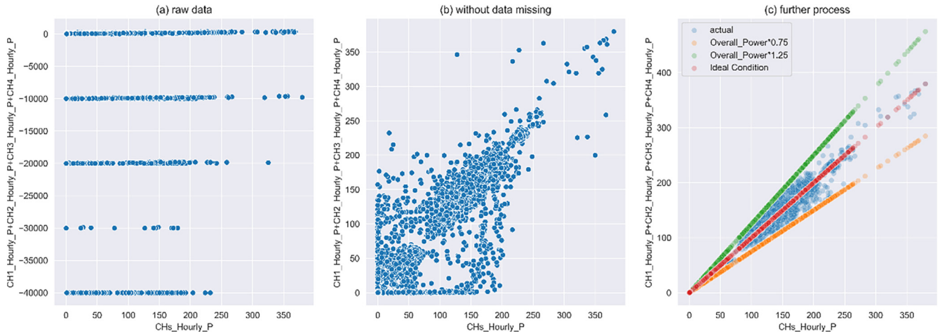
Fig. 10. The relationship between the summary of the hourly power of every chiller and the overall hourly power of all chillers. (a) raw data. (b) data without data missing. (c) after Kirchhoff's law.
